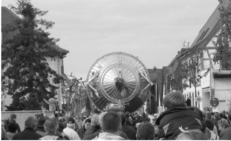
Figure 17. Transport of main spectrometer vessel through village of Leopoldshafen near FZK. At the narrowest point there was only a few centimeter clearance to the houses.
